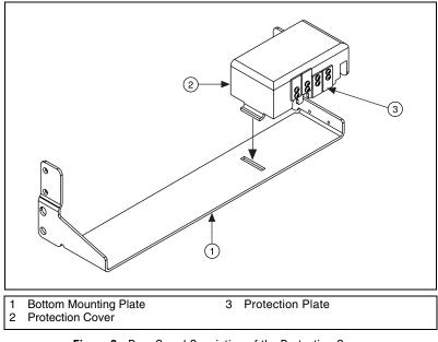
**Figure 9.** Rear Guard Consisting of the Protection Cover, Protection Plates, and Bottom Mounting Plate
